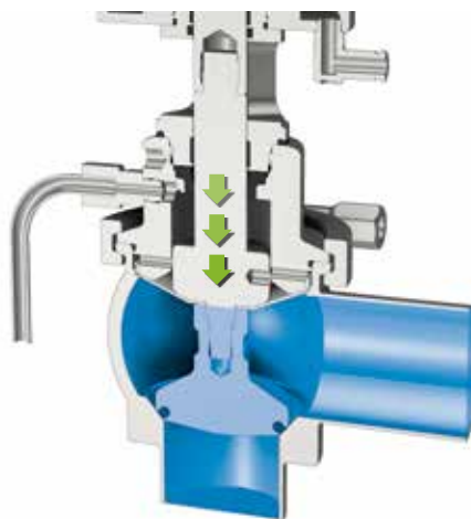
The aseptic barrier prevents the shuttle effect
