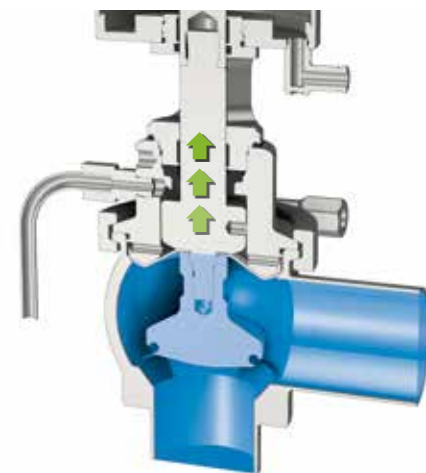
The aseptic barrier prevents the elevator effect
