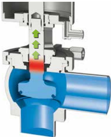
Elevator effect: When the valve is opening, product sticking onto the stem can be carried over behind the profile seal
