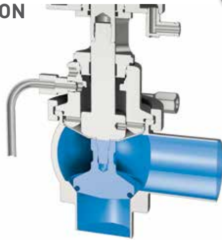
The P 3 diaphragm provides an aseptic barrier between the product area and atmosphere
